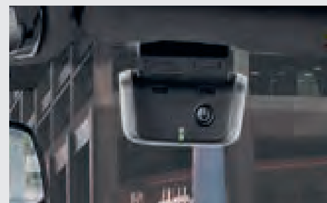
Advanced Car Eye 2.0. A highly sensitive full-HD camera that captures events in front and behind the car, even when it is parked. In the event of disturbances and extraordinary movement outside the vehicle, the camera automatically records the situation in order to document possible accidents or (attempted) break-ins.
