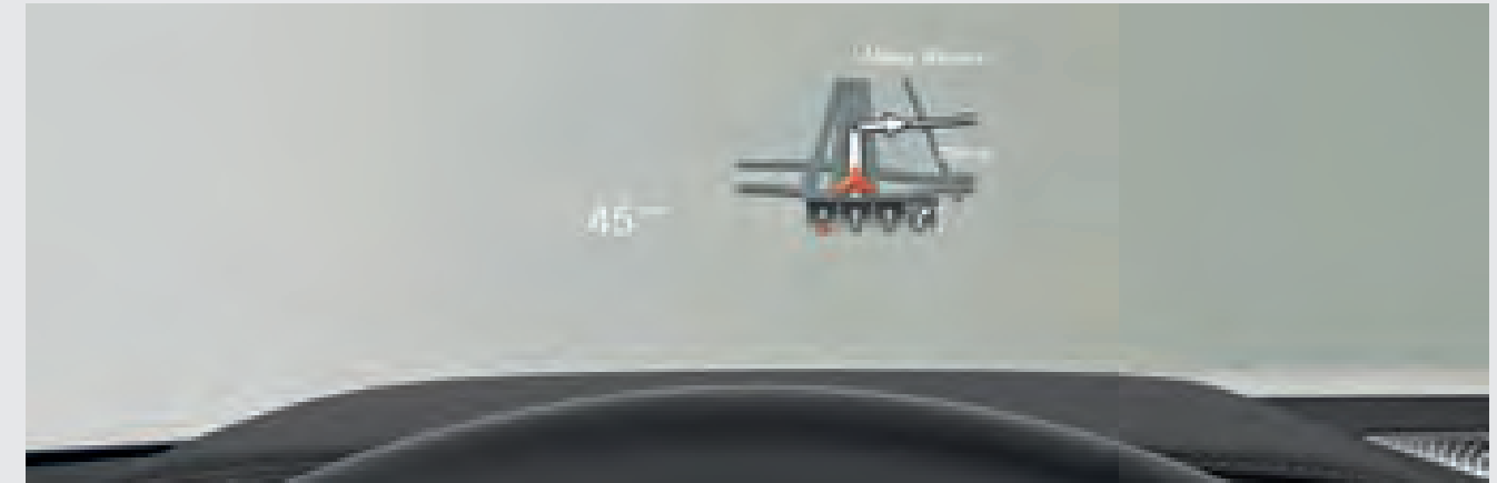
The full-colour BMW Head-Up Display projects all information relevant to the journey directly into the driver's field of vision, thereby allowing him to fully concentrate on driving. Information such as the current speed, navigation directions, along with telephone and entertainment information is displayed.
