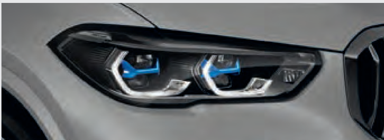
In laser high-beam mode, BMW Laserlight with X Signature illuminates a range of up to 600 m, nearly twice as far as that of conventional headlights. Better visibility in the dark significantly increases safety. The blue X signature and the "BMW Laser" lettering underline the vehicle's technological standards.
