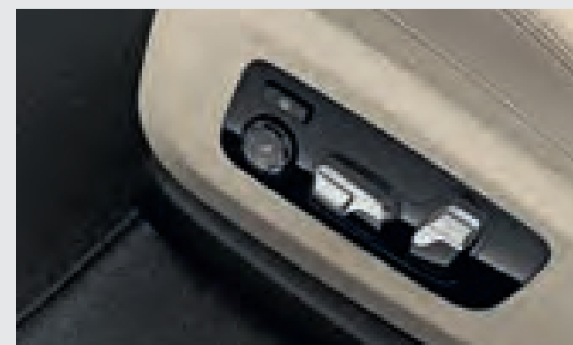
The Lumbar Support for the driver and front passenger seats can be adjusted both vertically and laterally, allowing for an orthopaedically optimised seating position.
